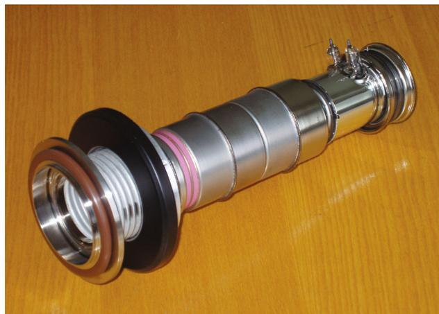
Fig. 7. The appearance of the PV-204XM X-ray EOC with an open entrance.
